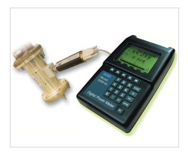
Bird® Electronic Corporation now offers a convenient, cost effective product for RF Power Measurement in High Power applications. The Bird BroadBand Directional Coupler uses the Bird Model 5000-EX, a handheld meter, with a Wideband Coupler and the Bird Terminating Power Sensor for accurate, repeatable readings of both UHF and VHF, forward and reflected power in broadcast facilities.
